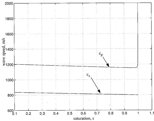
FIG. 1. Compressional and shear wave speeds computed from Eqs. (28), (29) and (32) to (35). The following parameter values, appropriate to the Murphy's Massillon sandstone, were used:  $N=0.23$ ;  $\rho_s=2660 \text{ kg/m}^3$ ;  $\rho_a=1 \text{ kg/m}^3$ ;  $\rho_w=998 \text{ kg/m}^3$ ;  $\kappa_s=3.6 \times 10^{10} \text{ Pa}$ ;  $\kappa_a=1.16 \times 10^5 \text{ Pa}$ ;  $\kappa_w=2.19 \times 10^{10} \text{ Pa}$ ;  $\bar{k}=0$ .
