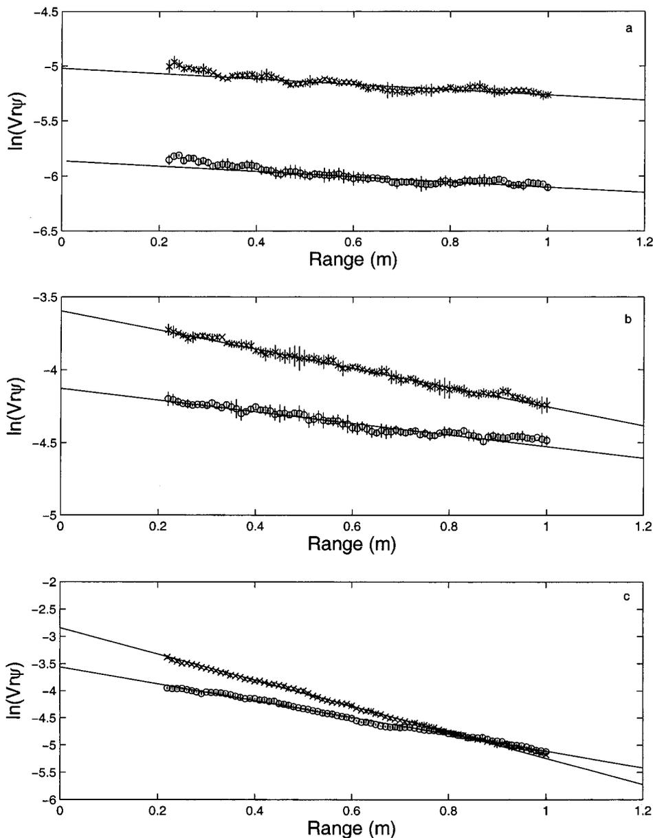
FIG. 6. Measurements of the variation of  $\ln(Vr\psi)$  with range,  $r$ , from the transducer at (a) 1.0 MHz, (b) 2.0 MHz, and (c) 4.0 MHz, for sand suspensions with  $\langle a_s \rangle = 57.75 \mu\text{m}$  ( $\circ$ ) and  $\langle a_s \rangle = 137.5 \mu\text{m}$  ( $\times$ ).
