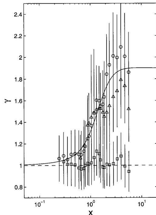
FIG. 8. Measurements for sand of the ratios  $f_x/f_s$  (○) and  $\chi_x/\chi_s$  (△) versus  $x$ , and Eq. (7) (—) with  $\beta=1.9$ . The equivalent calculation for the glass sphere results are given by (□).
