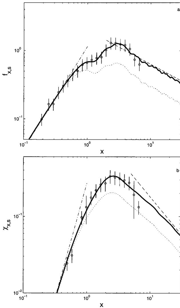
FIG. 11. (a) The variation in  $f_x$  ( $\circ$ ) obtained by combining all the measurement on sand suspensions. (—)  $f_s$  with  $\beta=1.9$ , ( $\cdots$ )  $f_s$  with  $\gamma=1$ . (b) The variation in  $\chi_x$  ( $\circ$ ) obtained by combining all the measurement on sand suspensions. (—)  $\chi_s$  with  $\beta=1.7$ , ( $\cdots$ )  $\chi_s$  with  $\gamma=1$ . (---) is Rayleigh scattering and (- -) is geometric scattering.
