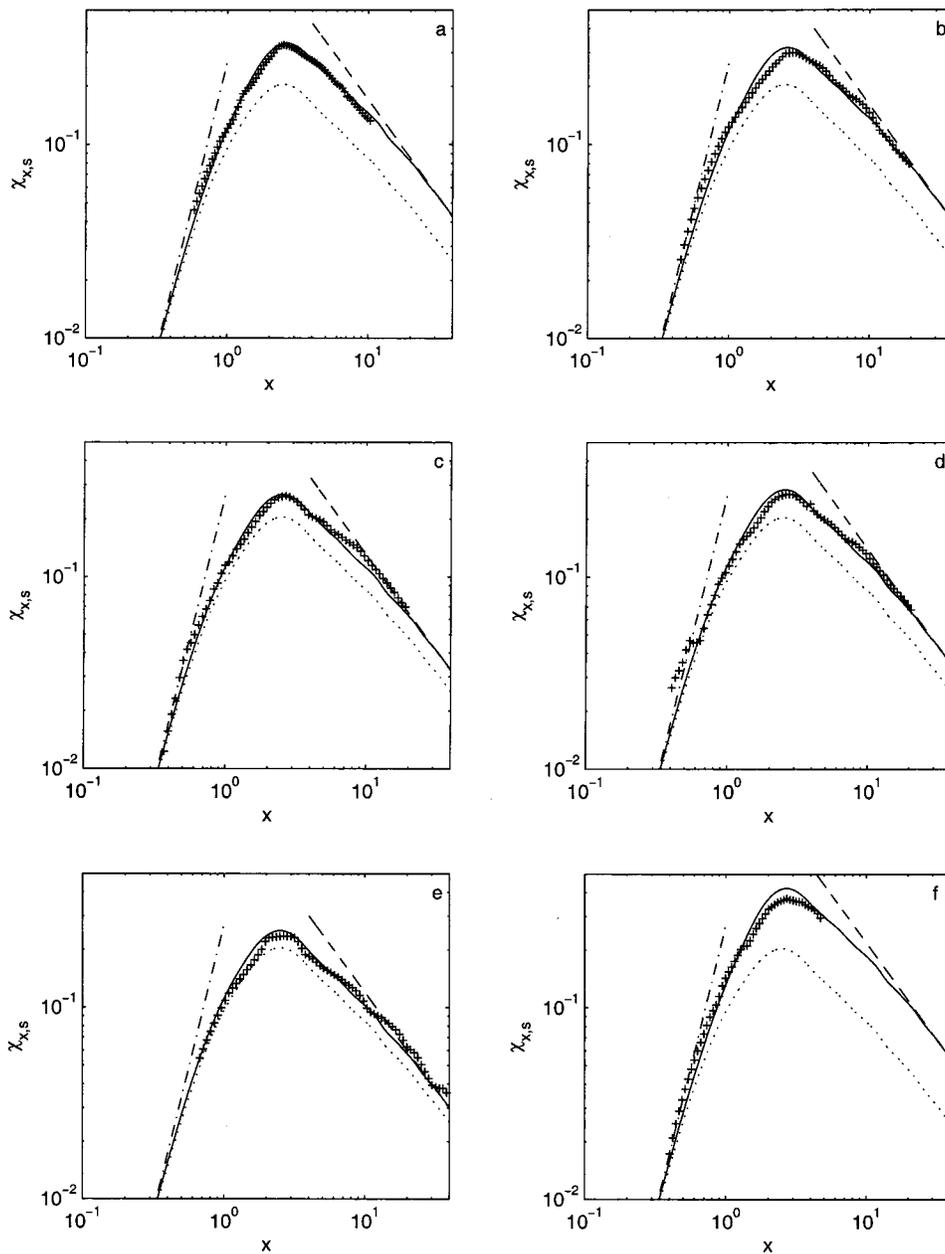
FIG. 12. Comparison of  $\chi_x$  (+) and  $\chi_s$  (—) for the sand suspensions of Ref. 5, ( $\cdots$ )  $\gamma=1$  in Eq. (5b), (---) Rayleigh scattering and (-·-) geometric scattering. (a) Assen sand 1, (b) Assen sand 2, (c) Ottawa sand, (d) Twente sand, (e) dune sand and (f) quartz particles.
