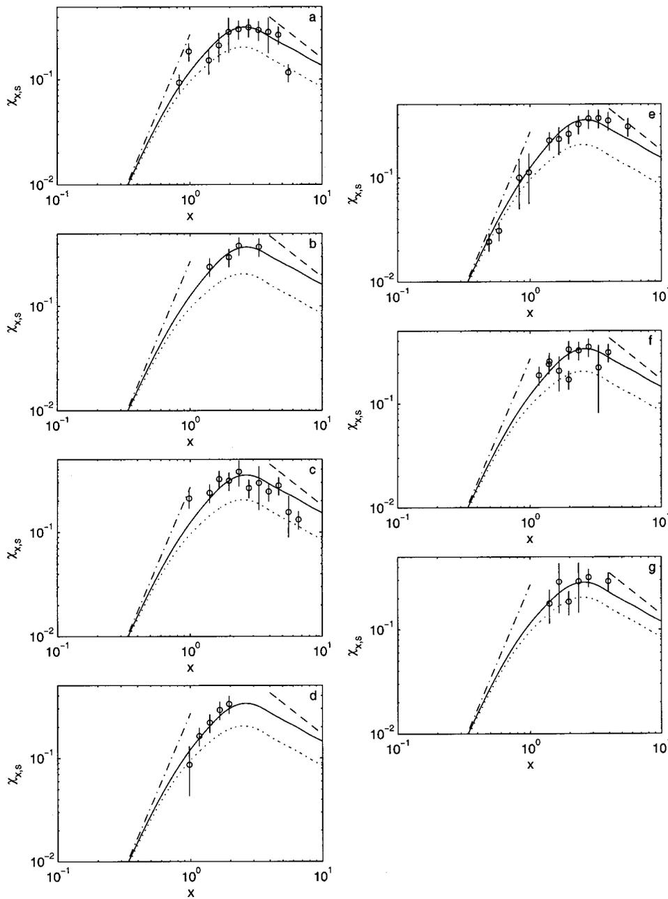
FIG. 10. Comparison of  $\chi_x$  ( $\circ$ ) and  $\chi_s$  (—) for all of the sand suspensions, ( $\cdots$ )  $\gamma=1$  in Eq. (5b), (---) Rayleigh scattering and (-·-) geometric scattering. In the present figure and the following, plots  $\chi_{x,s}$  represents  $\chi_x$ ,  $\chi_s$ .
