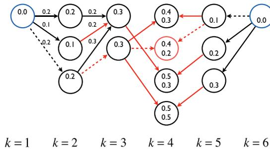
Figure 1: The nodes represent detected peaks at different transmission times  $k$ . The arrows represent transition costs between nodes. The total cost of a path from the left/right is the sum of the costs along the path and is shown in the top/bottom number at a node. The most likely node at a particular time is the one with lowest total costs.
