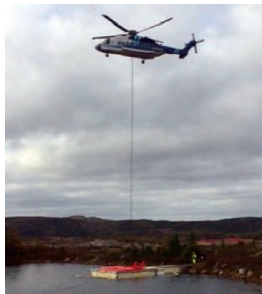
Figure 46. Test of an airborne earth-field NMR system for detecting near-surface contaminants. Image courtesy of ExxonMobil.
