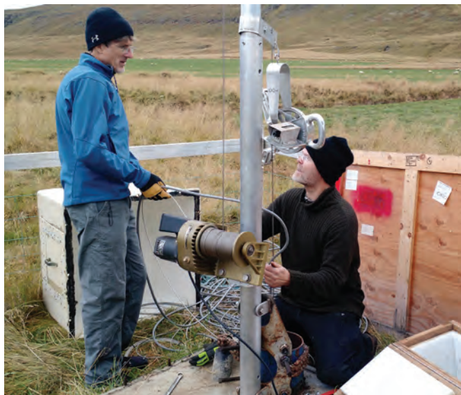
Figure 16. Dr. Carl Ebeling (left), IDA's chief engineer, and Bergur Bergsson (right) of the host Iceland Meteorological Office carefully lower a new seismometer package into the borehole at GSN station BORG (Borganes, Iceland).
