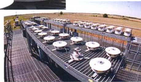
Above, Radiometers measure solar infrared radiation.
