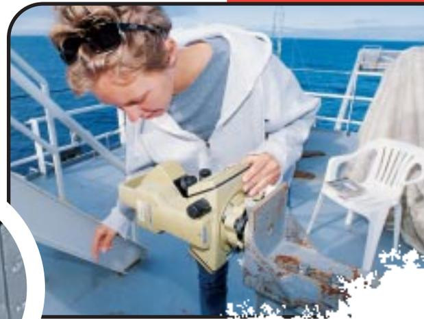
*Above, Nicole Olivares, a UCSD student, uses a survey instrument to position the GPS antennas with the acoustic transducer that is lowered through a hole (left) to extend beneath the ship's hull (bottom, opposite page).*
