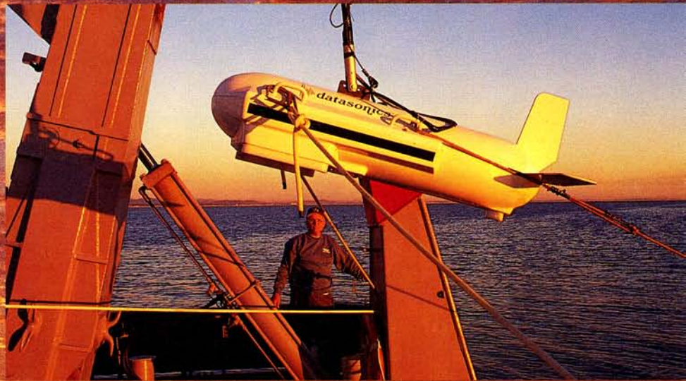
A towed mapping instrument, called a fish, is brought aboard R/V Melville ; veteran Scripps oceanographer Robert Fisher observes in the background.
