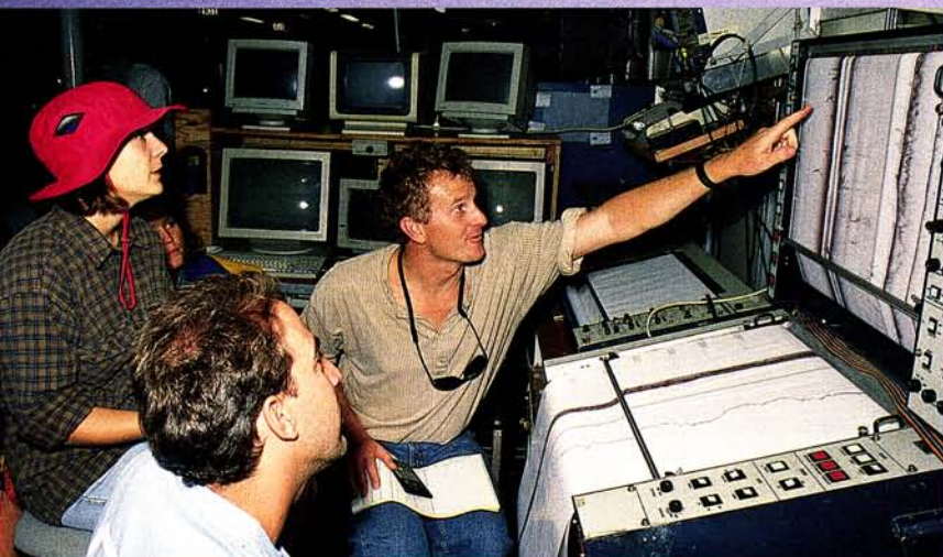
In the ship's well-equipped computer lab (above), Kevin Brown points to a specific seabed feature detected by a subbottom profiler. At the beginning of the cruise, Brown (upper right) reviews shift assignments during the first science meeting. Scripps associate specialist Allan Sauter (right) and volunteer Alan Trujillo prepare the fish for deployment.
