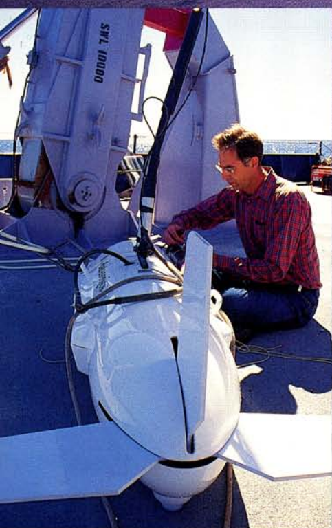
Sauter affixes an acoustic device to the fish, which will help determine the instrument's orientation in the water column.
