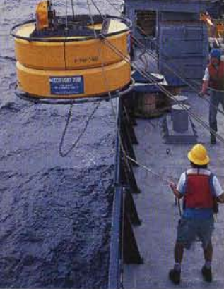
Above, (left to right), Suspended in the water column with subsurface floats, tomography arrays deployed by Peter Worcester determined velocity of tidal currents.
