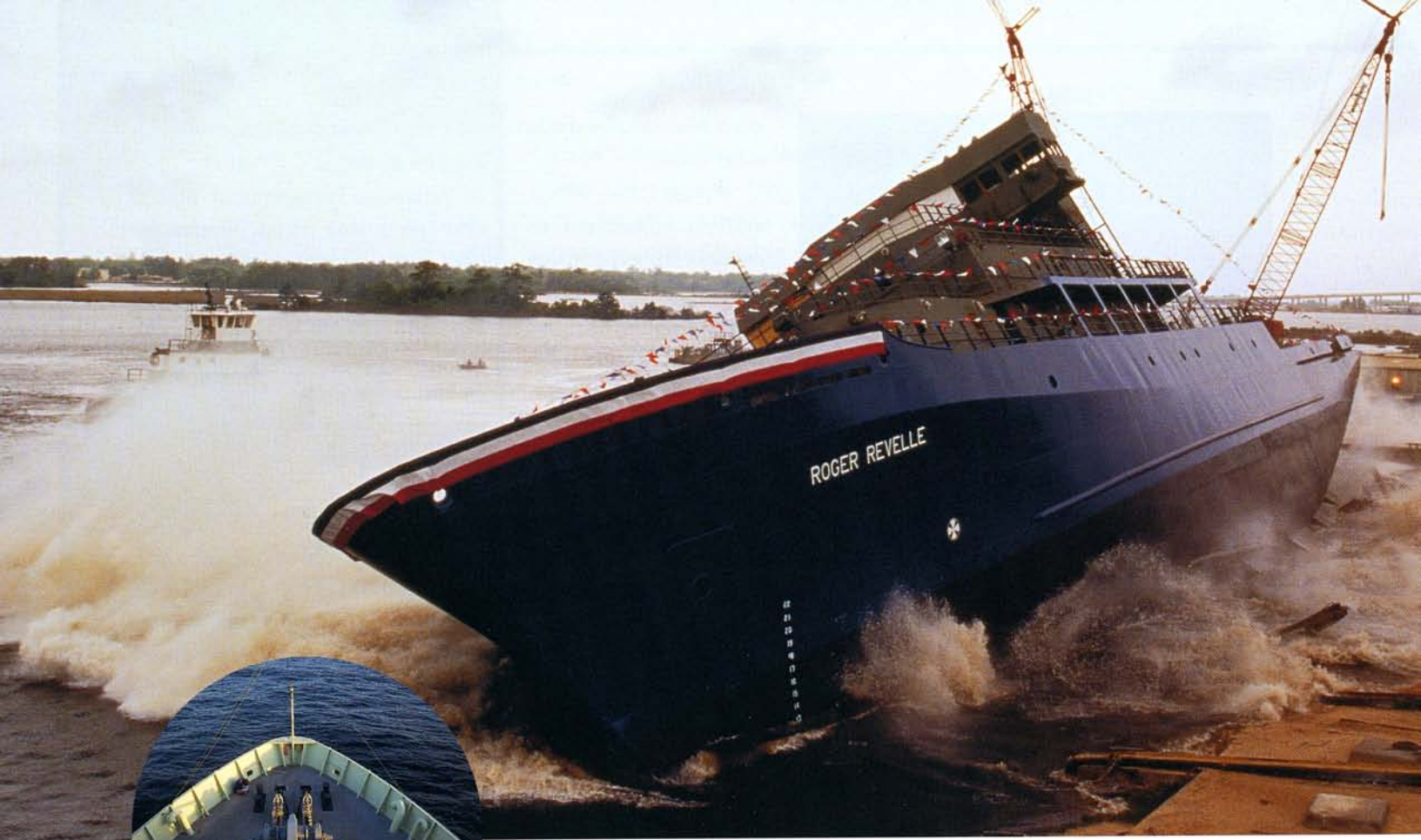
Above, The 275-foot R/V Roger Revelle being launched on the Mississippi River in 1996. It is among the largest and most capable of modern oceanographic research vessels.
