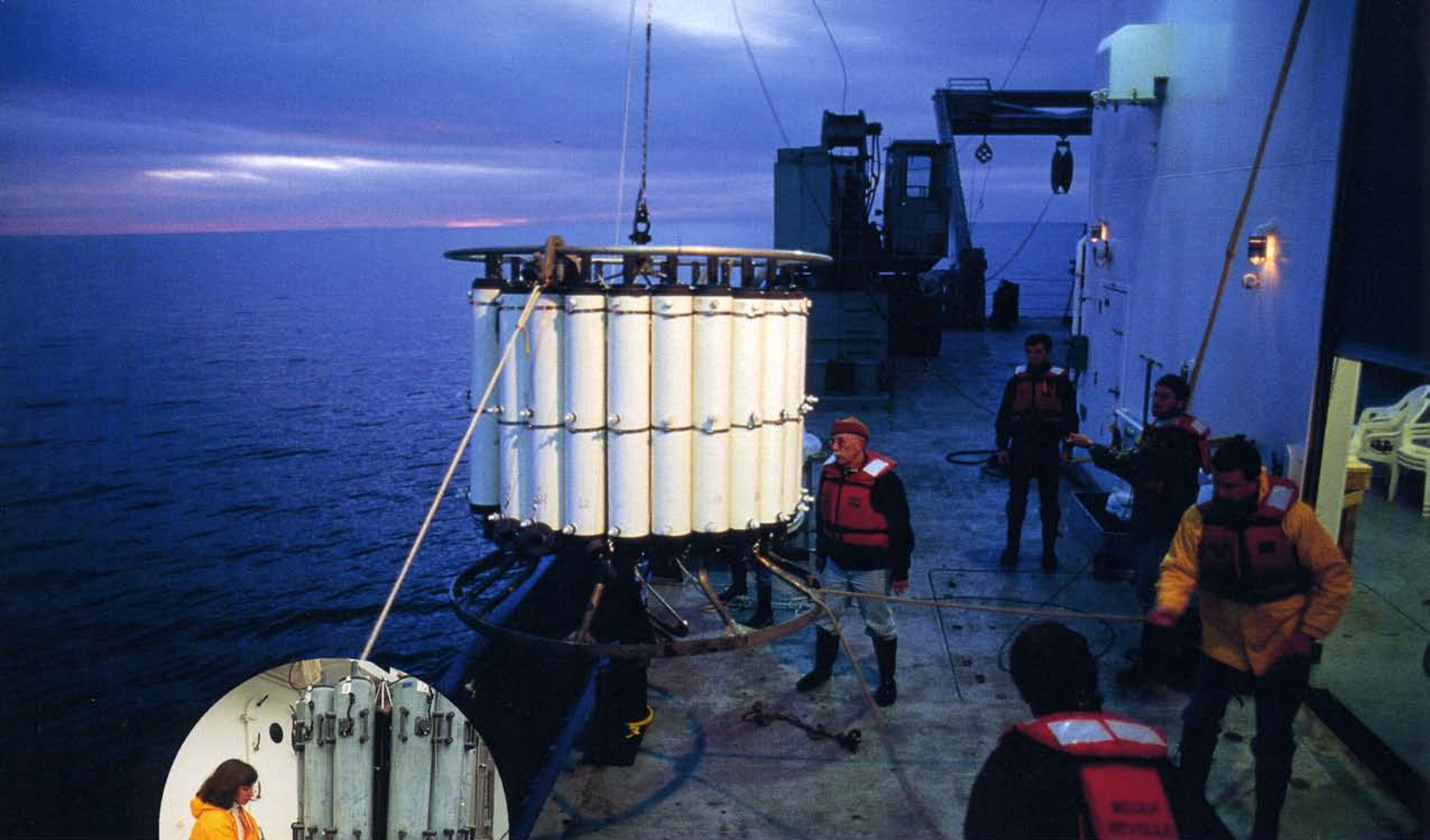
Above, Deployment of conductivity temperature density (CTD) casts containing water-sampling bottles used for measuring temperature and salinity at various ocean depths. Left, Physical oceanographer Lynn Talley draws a water sample from a CTD rosette during the World Ocean Circulation Experiment.
