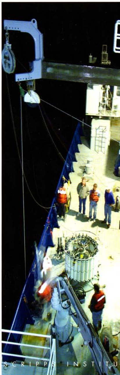
Opposite page , A CTD rosette is prepared for deployment. Above , Marine geochemist Lihini Aluwihare, with student Roman de Jesus (below), studies the role of dissolved organic matter in the California Current.
