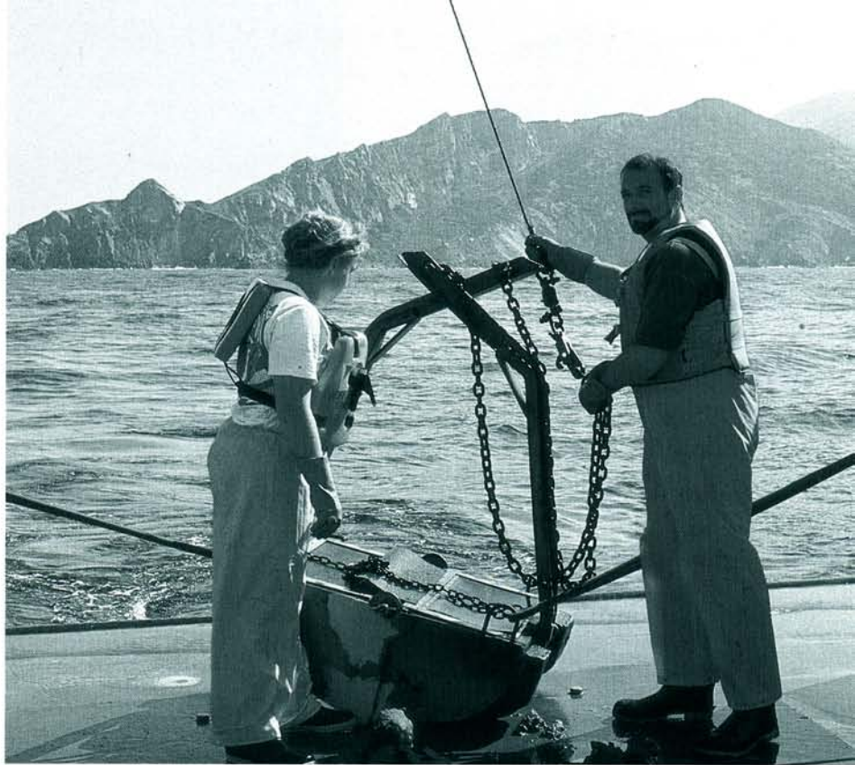
The Van Veen grab is very heavy, tricky to maneuver, and requires a coordinated effort. Graduate student Karen Casciotti and Richard Cosson, a researcher from France, prepare to open the grab.
