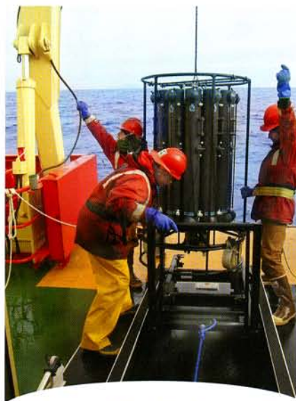
Chris Measures (left) and his University of Hawaii team deploy a water-sampling rosette for trace metal studies.
