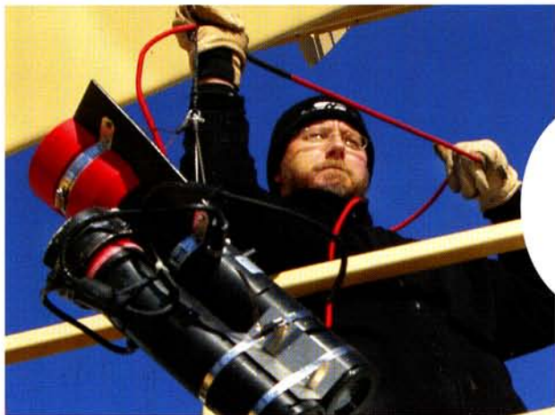
Top, Rick Reynolds recovers an instrument for measuring the optical properties of the upper water layers. Bottom, Bottles in the ship's "Antarctic Tanning Salon" contain water samples enriched with iron that will be used to analyze phytoplankton responses. The artificial light mimics the wavelengths of sunlight.
