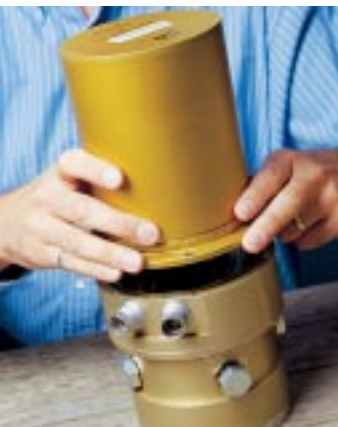
Left and above, Hedlin shows off a microbarometer, inside and out.
