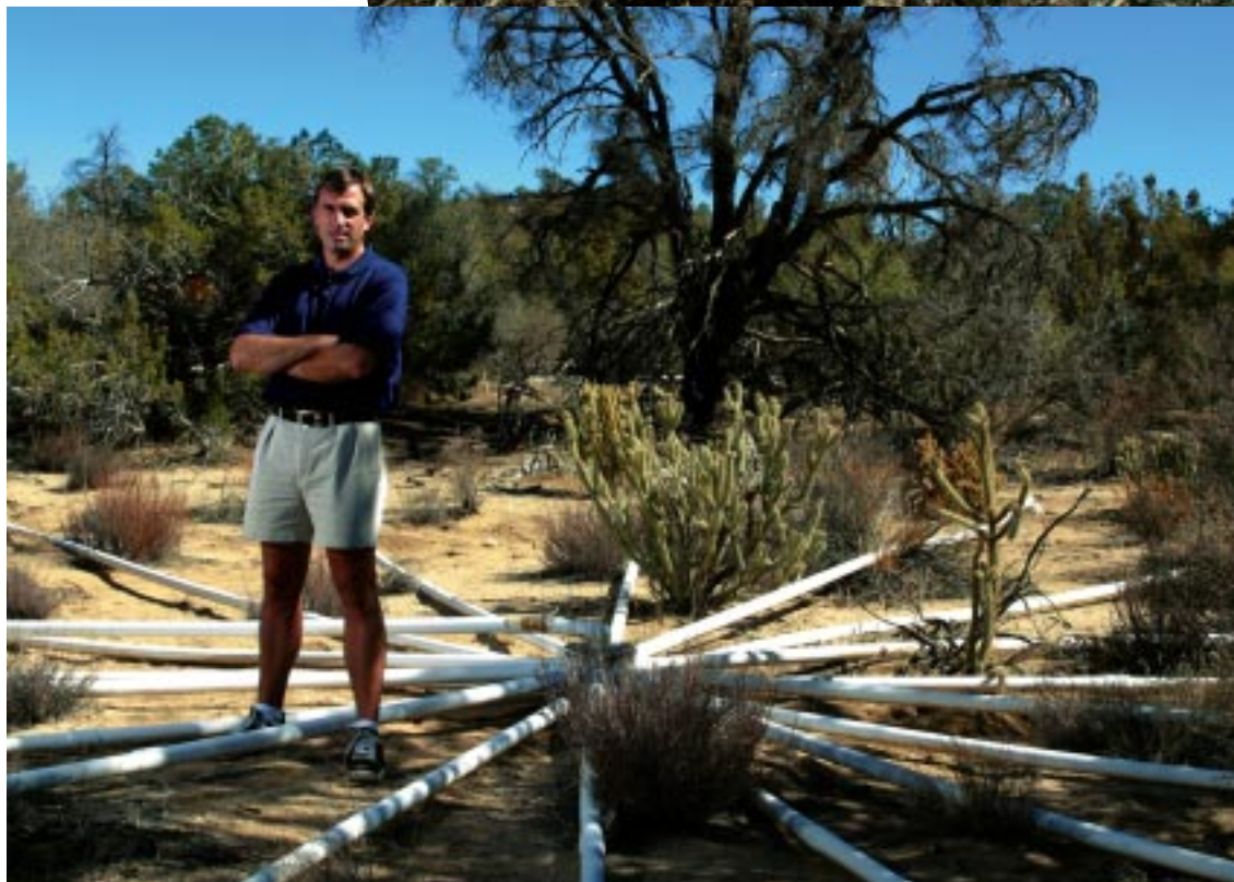
This page, In the brush-covered desert south of Palm Springs, a Scripps microbarometer element is identified by its distinctive spokelike sound filters.
