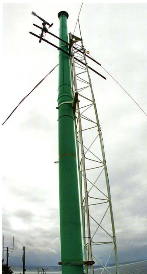
Above, Salt from the relentless sea spray of the northern California coast was a common input for ATOFMS, which took in air through an aerosol mast (left) built to minimize contamination from local land-based sources.
