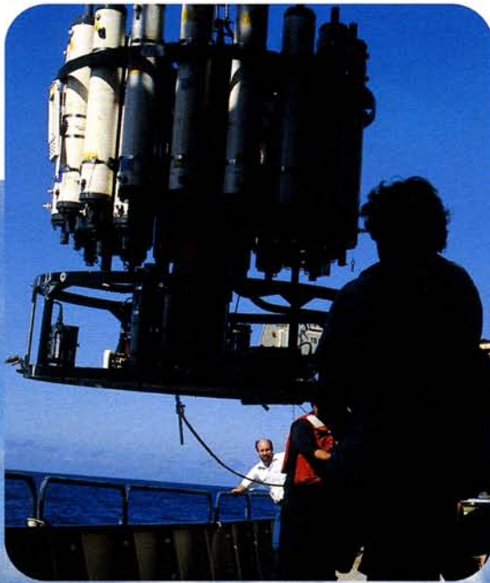
A CTD rosette is carefully lowered into the water while Wells (in baseball cap) and others monitor its progress. Inset , A rosette holds many individual data transmitting devices.
