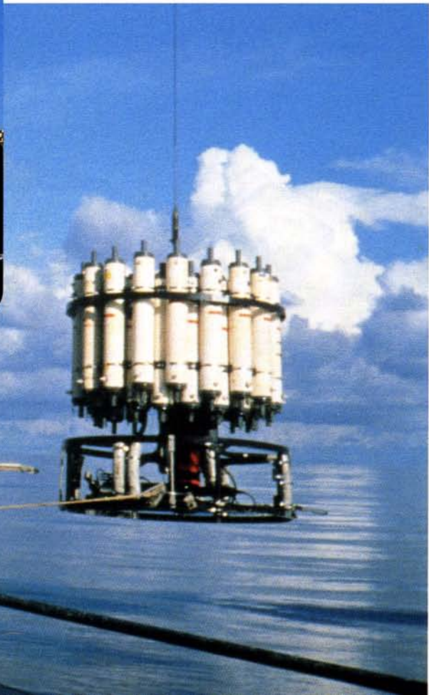
A CTD rosette is carefully lowered into the water while Wells (in baseball cap) and others monitor its progress. Inset , A rosette holds many individual data transmitting devices.
