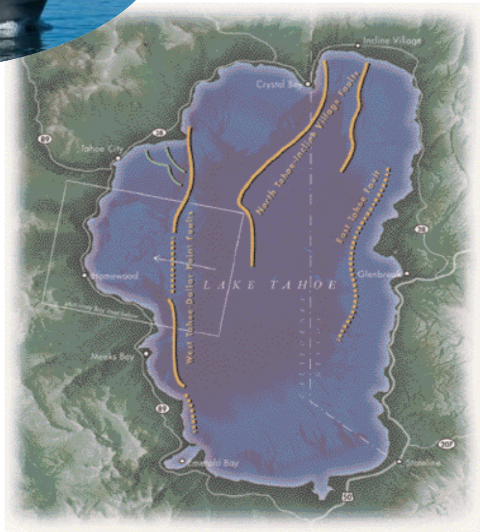
Above, This United States Geological Survey bathymetry map highlights Lake Tahoe's largest fault lines, which represent a significant risk of triggering tsunamis through ground movement and landslides. The box outlines an area of collapse at McKinney Bay (see detailed image on page 11).
