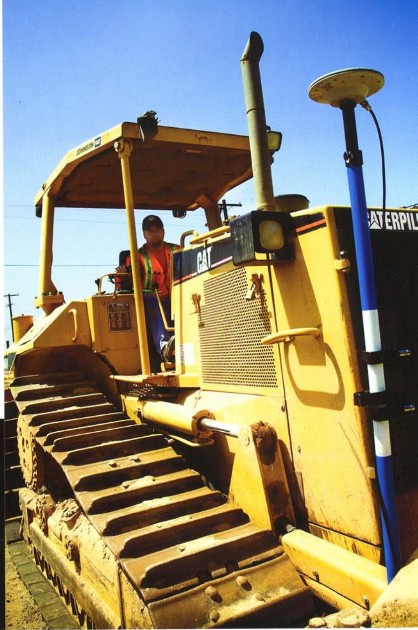
Right, A GPS antenna mounted on a tractor is an example of how GPS technology is being used for a variety of real-time applications.
