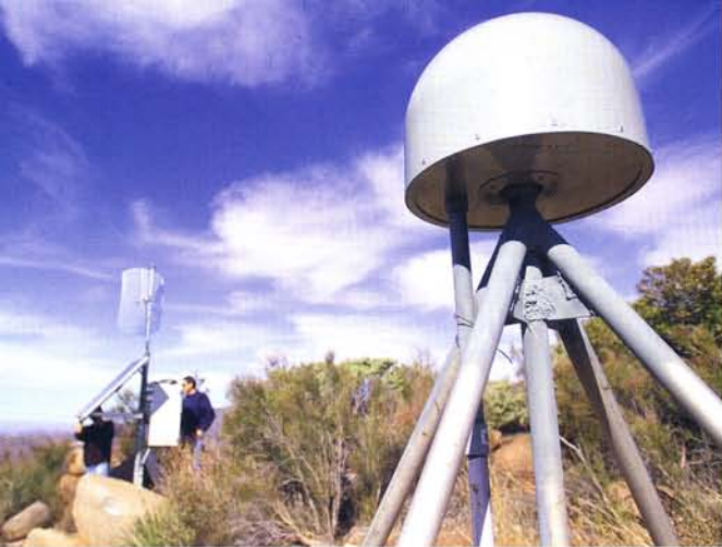
Above, San Diego County completed a real-time GPS network with this receiver installed in Descanso in spring 2006.
