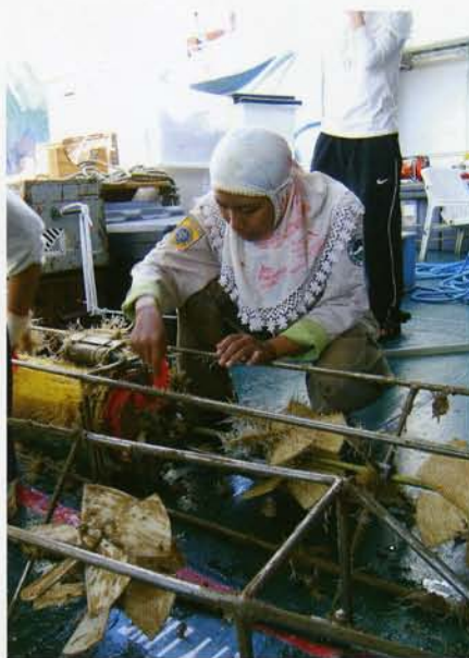
Above, Clearing a seaweed-coated rotary current meter during INSTANT. Opposite, Janet Sprintall back at Scripps with a cleaner version.
