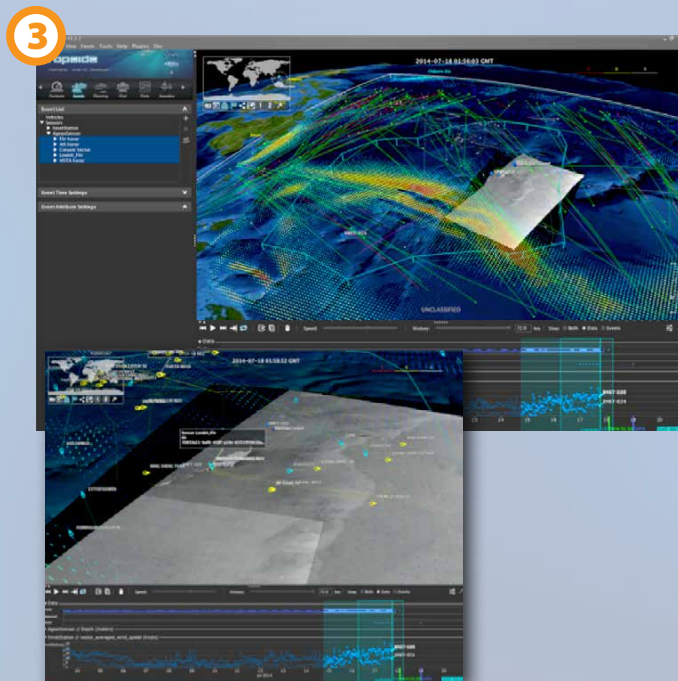
(top) Data fusion of AIS and legal fishing boat tracks overlaid with ocean circulation forecasts and commercial Synthetic Aperture Radar (SAR) image. (inset) Zoomed region of SAR image, AIS tracks, and identified "dark" targets potentially engaged in IUU.
