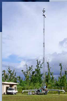
(above) Nested concept of operations showing data flow. Two PGST towers were employed during the MDA demonstration, one on Kotor (due to topography, full 360° coverage was not available), and one on Kayangel (top middle full yellow circle). (right) Shore-based tower on Kayangel with radar, sensors, and satellite communications systems.
