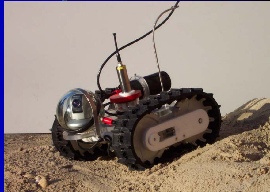
UW Crawler with pan&tilt video camera (VENUS)
