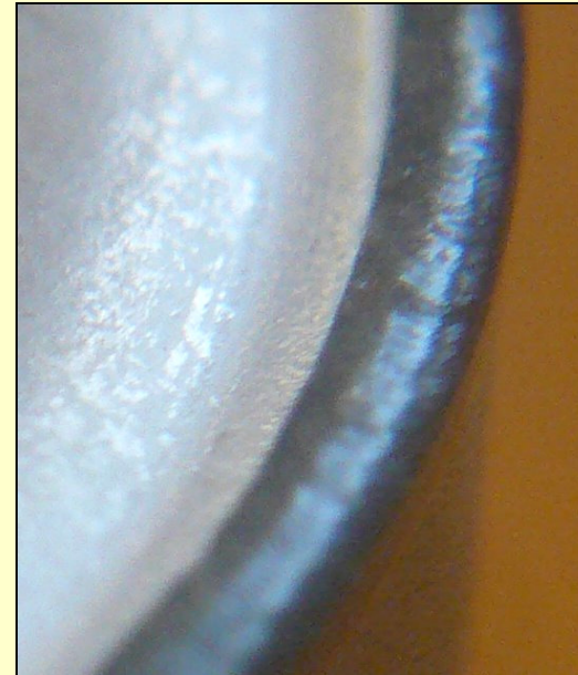
Laser weld between lid and can
