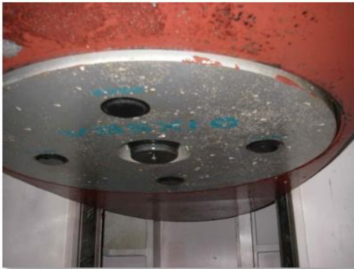
Flush antenna installed on R/V Sarmiento do Gamboa, CSIC Spain. The antenna is on a sliding gondola deployed on request
