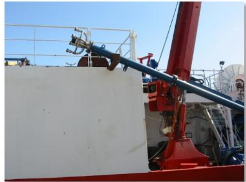
Deployage antenna on pole onbaord Svitzer Mercator, UK
