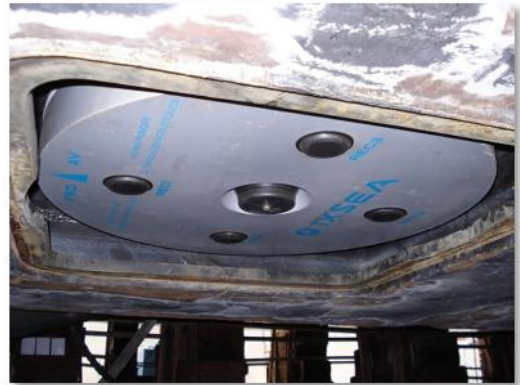
Flush antenna installed on R/V Polarstern / AWI Germany a window can protect the antenna in very icy conditions
