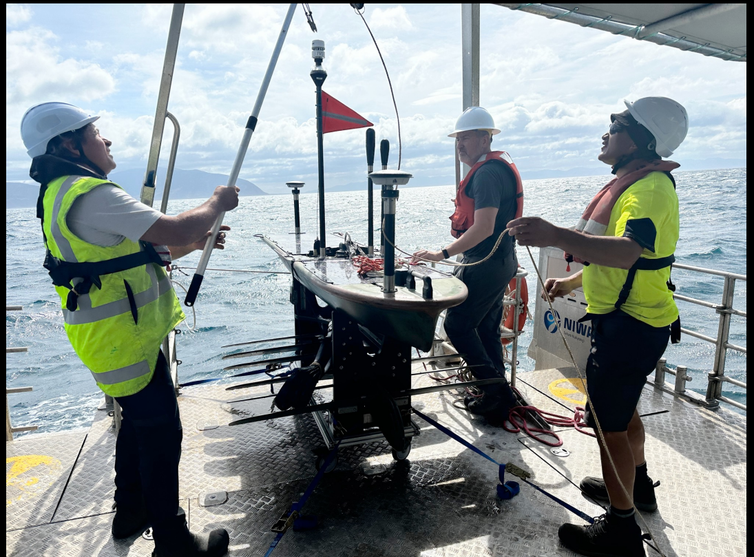
wave glider launch offshore New Zealand for GNSS-Acoustic survey
